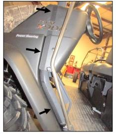
**1.** Adhere Velcro strips to lower front corner the vehicle as shown.
