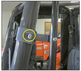
**2.** Loosely attach the front of the subframe to the clamp on the front of the vehicle using a M6 x 20mm bolt, nut and 2 washers.
