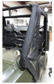
**3.** Remove bar & Install side panels to the front roll cage bars correctly.
