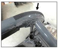
**6.** Adhere Velcro straps to upper front corner the roll cage as shown. They should line up with the Velcro on the fabric.
