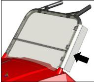
This is preferred method. Best used for 2pc., folding, & 1/2 windshields. Side Panel Velcro's directly to Roll Bar. Notches are cut into side panel to accommodate mounting system. Minimizes interferences with 2pc. & folding windshield functions.
