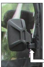
Install mirror with supplied hardware. Adjust position as required.
