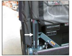
**5.** Adhere Velcro strips to the rear roll cage in the position shown. They should line up with the Velcro on the fabric.
