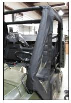
1. Mount side panel cab sections positioned correctly & taught.
