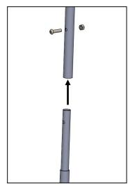
**2.** Attach the Upper Subframe (A) to the Lower Front Subframe (B) with a M6 x 25mm socket head bolt and nut.
