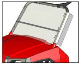
2. Lay the windshield in position noting location of the slots where the mounting straps will go NOTE: You will cut the side panels - Ensure they are positioned correctly.
