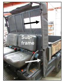
**4.** Wrap the subframe textile around the rear subframe and attach using velcro on the fabric.
