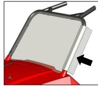
This method is best for full 1pc windshields where user doesn't plan on switching it out after install as Velcro will adhere directly to windshield edge surface. It increases seal slightly but installation is a bit trickier. The surface to adhere the Velcro must be cleaned well, but alcohol should not be applied to acrylic or polycarbonate.
