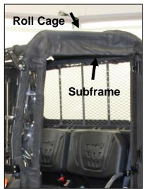
**6.** Wrap the subframe textile around the subframe and roll cage. Attach using velcro on the fabric.
