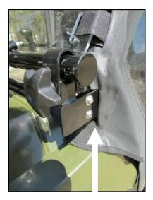
The side panel textile needs to be cut to accommodate the hood rack roll cage clamp / brackets.
