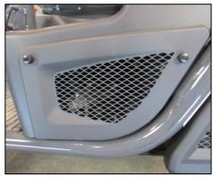
4. Reinstall the factory mesh panel.
