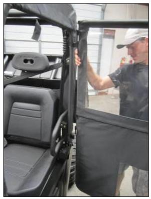
**5.** Mount the doors by guiding the pins in the back of the door frame onto the hinge barrels along the Door Hinge Subframe.
