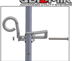
**2.** Assemble the door handle in the order shown above with the  $\frac{1}{4}$  - 20 x 2.5" Bolt and nut. Place the metal washers and plastic spacers between door and inside door handle. You may have to adjust the number of washers and spacers so the door closes against the subframe securely.
