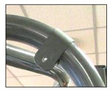
**2.** Place a clamp on the upper rear corner of the roll cage as shown above.
