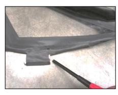
6. Mend the cuts with a lighter. Hold the flame on the material edge just long enough to melt the edge slightly. This will prevent the material fraying over time.
