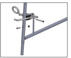
1. Place the door handle in place. The circular loop should be on the inside of the door.
