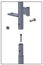
**3.** Attach the Door Hinge Subframe (C) to the Lower Rear Subframe (D) with a M6 x 25mm socket head bolt and nut. The hinge will be on the back side of the tube.
