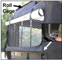
**2.** Hook the bottom of the back panel to the bottom of the rear bar. Then strap the top across the upper rear roll cage crossbar.
