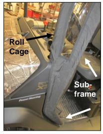
**3.** Wrap the subframe textile around the front subframe and roll cage and attach using velcro on the fabric.
