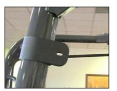
**1.** Place a clamp on the front roll cage bar. Refer to the picture below for locations.
