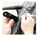
**4.** Reinstall side panels, verify light bar clamp position & mark fabric
