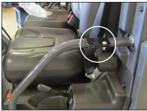
**7.** Place the door hinge bar clamp about 4 inches away from the end of the bar. Loosely attach with a single M6 x 20mm hex bolt, two washers and nut in the rear hole as shown above.
