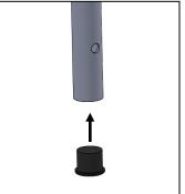
**4.** Push End Plug (J) into end of the tubes.
