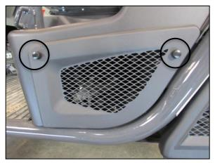
**7.** Remove factory mesh panel under the seat by loosening the two plastic thumb screws shown above.
