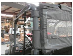
**1.** Attach the back panel by strapping it to the rear vertical roll cage bars on both sides.
