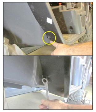
**5.** Locate and remove this bolt in the front wheel well.
