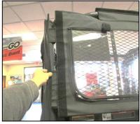
**5.** Attach the subframe textile to the velcro strip on the back panel.
