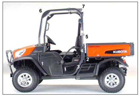
In the next few steps, you will be installing self adhesive velcro on the vehicle in the positions shown. Clean all surfaces with rubbing alcohol before installing Velcro Strips
